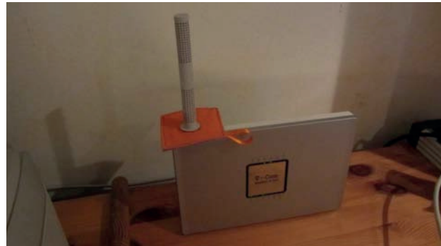
Antenna at router with attenuation sleeve
