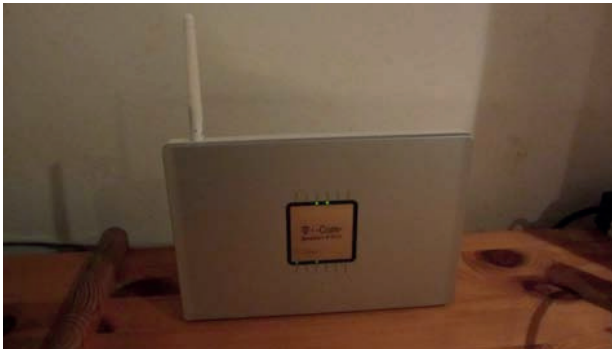
Antenna at router - not shielded
